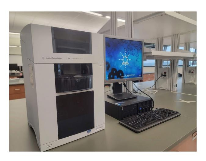
Model: Agilent capillary electrophoresis 7100
